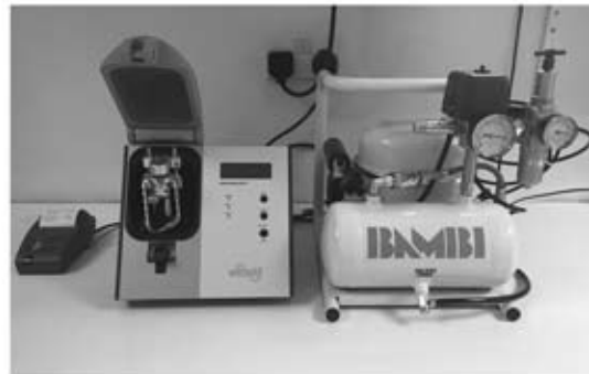
Witschi Proofmaster S to test the water resistance of watches.
